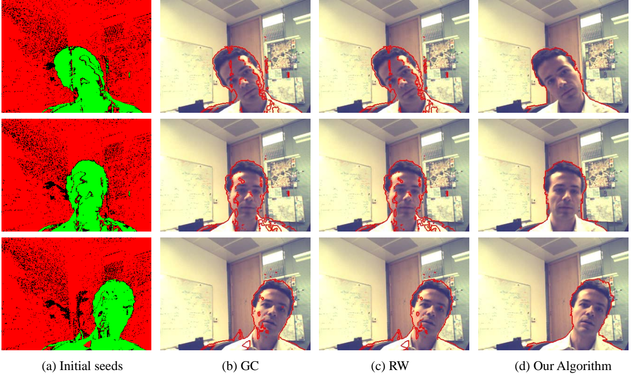
Fig. 4: Comparison of our algorithm with GC and RW on ‘A_anto’ sequence (200 frames) [8]. (b),(c) and (d) are the segmentation results of GC, RW and our algorithm, respectively. ( c = 0.0002 )
