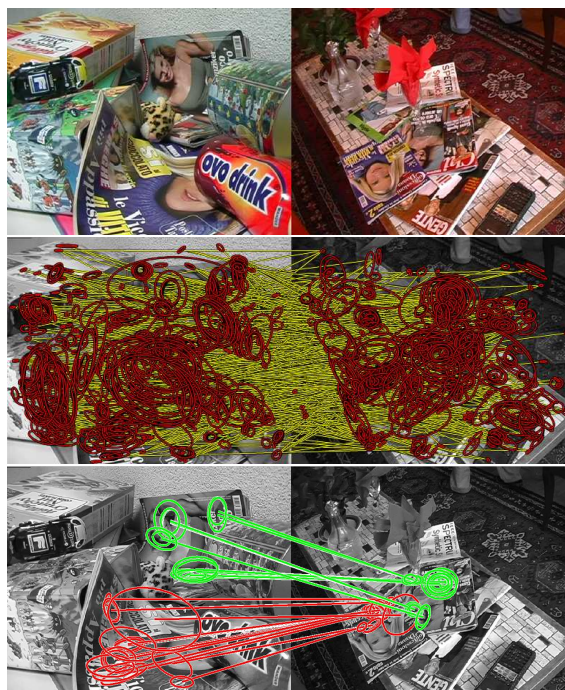
Figure 1. A result of our object-based image matching. It establishes both feature correspondences and their object-based clusters across arbitrary image pairs. Despite deformation of objects and high outlier ratio of candidate feature matches as shown in the middle, our method extracts multiple clusters of reliable matches, each representing a geometrically distinctive group of matches. It enables object-based image matching as shown in the bottom. Two detected clusters of feature correspondences are colored in red and green, respectively.
