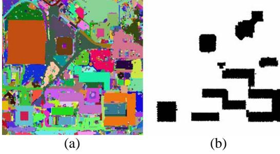
Fig. 2. Extracting coarse building region. (a) Segmentation result by mean-shift method, (b) Detected building region from LiDAR data
