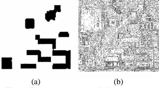
Fig. 4. Extracting precise building region. (a) Coarse building region extracted from Fig. 2, (b) Detected edge by Nevatia-Babu edge detector
