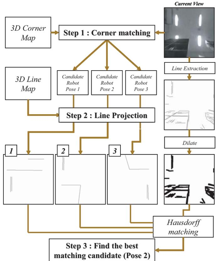
Fig. 5. Proposed relocation algorithm using both 3D corner and line landmarks
