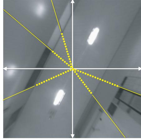
Fig. 3. Vertical line detection: All vertical lines vanish at the optical center
