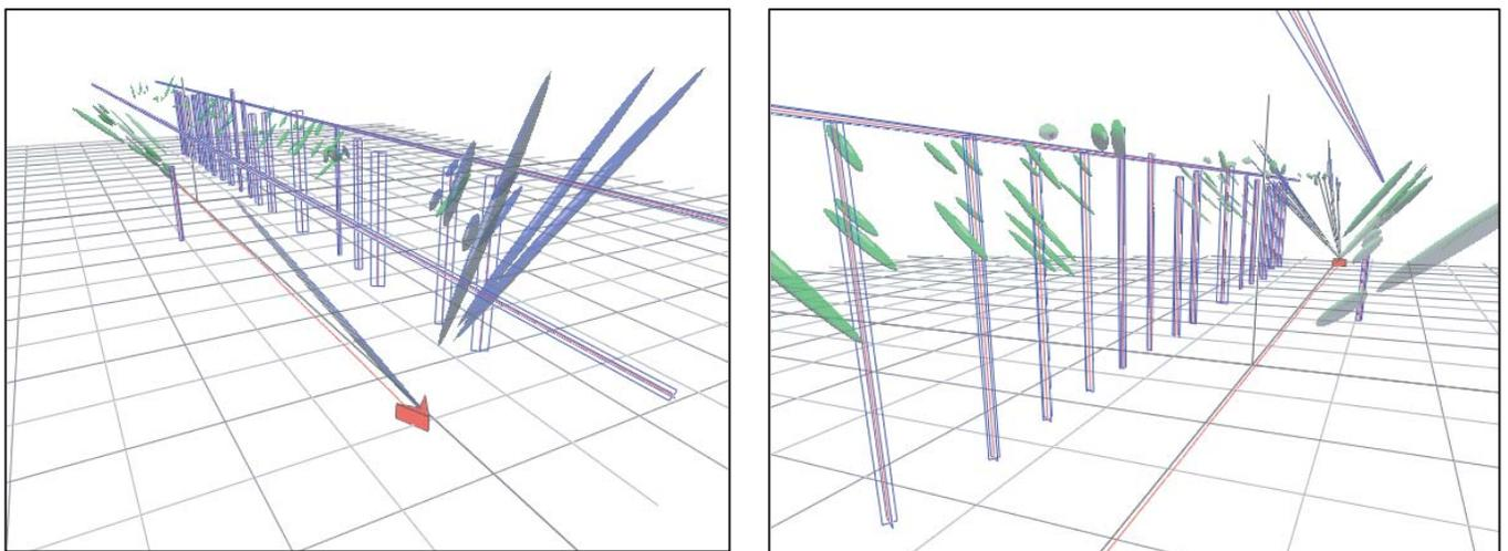
Fig. 9. Perspective views of the map building result by the proposed hybrid-landmark based SLAM
