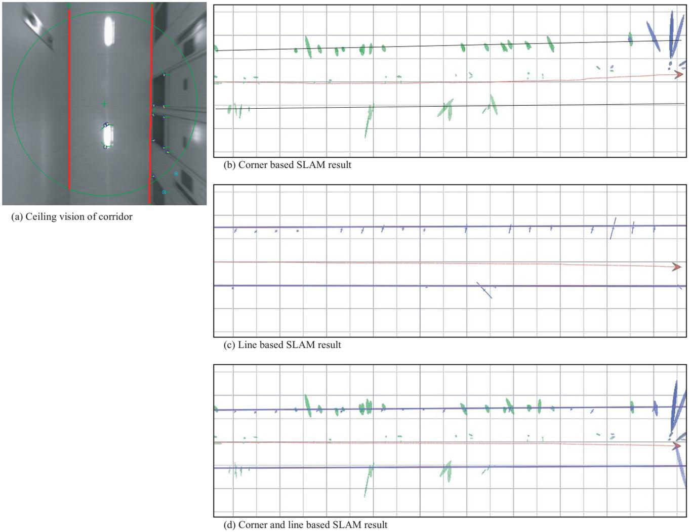
Fig. 8. Comparison of map building and localization results: results by (b) corner, (c) line, and (d) hybrid landmark-based SLAM technique for a test sequence of a long corridor shown in (a)
