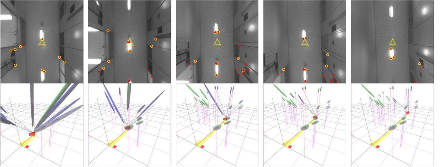
Fig. 10 Real time sequential map building experiment: corridor
