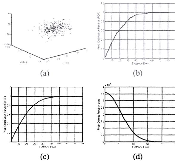
Figure 3. Error modeling of the range finder (a) Error distribution at the reference points (b) Measured probability distribution function (c) Estimated Gaussian distribution function (d) Estimated Gaussian density function
