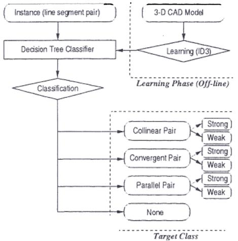
Figure 4. Block diagram of the classification using decision tree classifier
