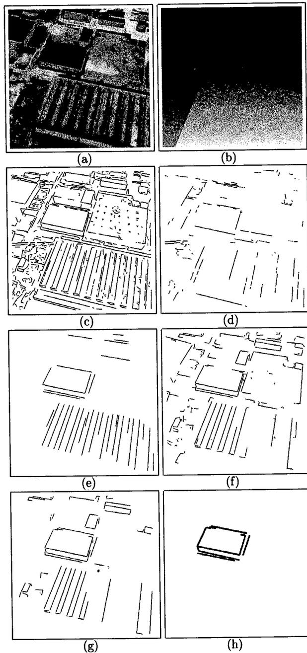
Figure 7: Multilevel grouping result (a) Input scene (from oblique view) (b) Depth image (c) Extracted line segments (d) Detected collinear pairs (e) Detected parallel pairs (f) Detected L-typed convergent pairs (g) Detected U-structures (h) Grouping result
