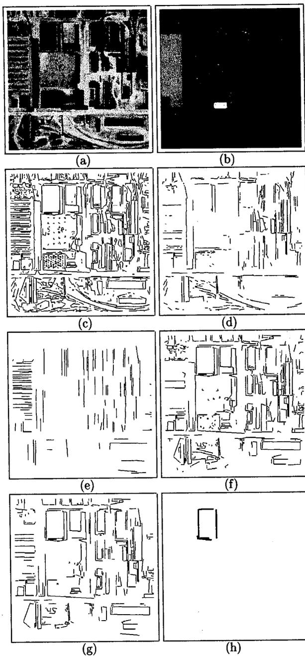
Figure 6: Multilevel grouping result (a) Input scene (from top view) (b) Depth image (c) Extracted line segments (d) Detected collinear pairs (e) Detected parallel pairs (f) Detected L-typed convergent pairs (g) Detected U-structures (h) Grouping result
