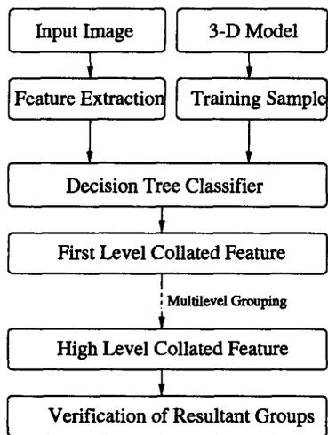
Figure 1: Block diagram of the proposed grouping procedure
