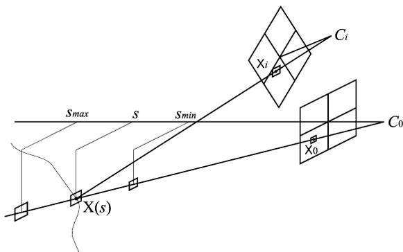
Fig. 1. General motion stereo camera model.
