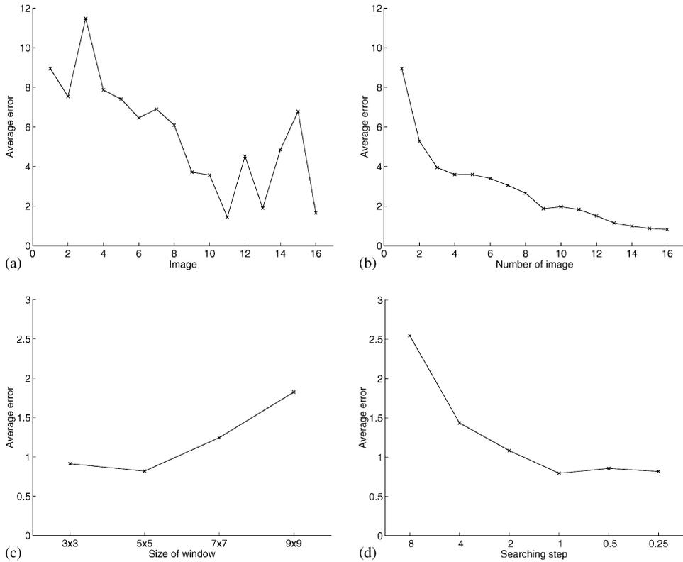
Fig. 9. Average error for the synthetic building images: (a) binocular stereo, (b) SWSSSD, (c) size of window, (d) searching step.
